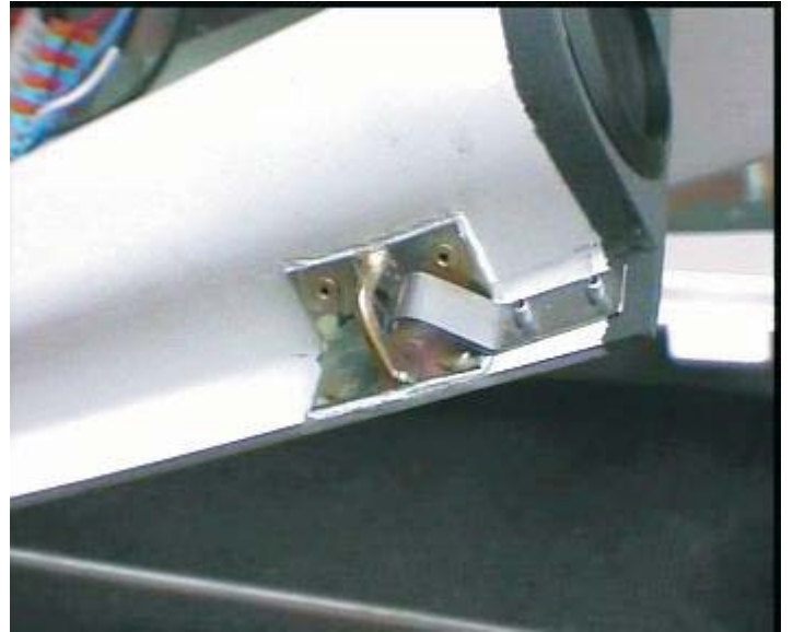
DETAIL OF AFT ACTUATING SPRING
