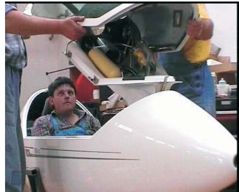
6. THE INSTRUMENT PANEL RISES TO PROTECT THE PILOT FROM INJURY
