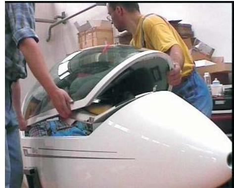
5. AFT PIVOT PIN HOLDS REAR EDGE OF CANOPY FRAME. THE AIR LIFT ONLY FRONT PART
