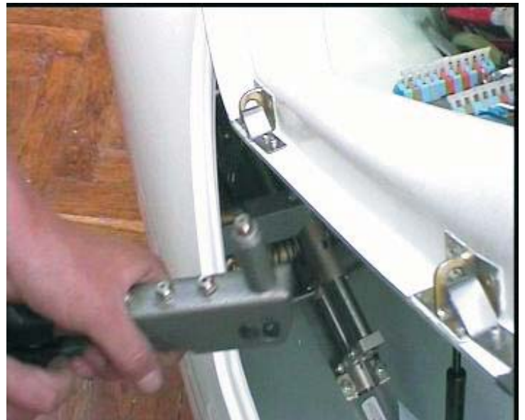
DETAIL OF ACTUATING SPRING - RIVETS IN INVERT POSITION
