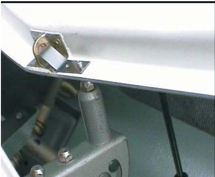
DETAIL OF ACTUATING SPRING - RIVETS IN INVERT POSITION
