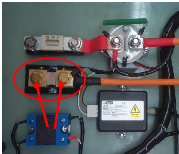
Figure 1 – Detail of shunt circuit (encircled, with screws marked with arrows)
