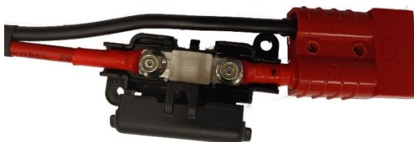
Fig. 3 – Fuse box detail.
